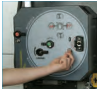
5 Unlock the air rotary isolator by the key (if available)
