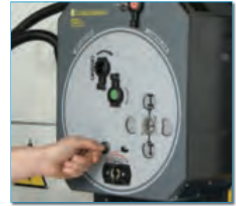
3 Unlock the air rotary isolator by the key (if available)
