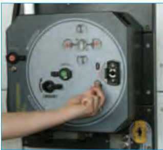
7 Lock the air rotary isolator by the key (if available)
