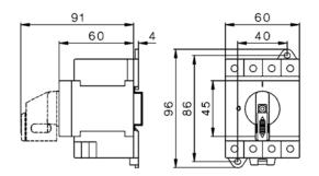
The construction of the switch ensures reliable switching up to 32A with 1000V in the category DC 21B.
