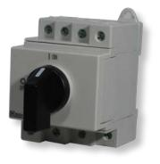
Switch disconnectors "LS.." are switch gears for interupting DC/AC-inverter from the solar-panels. Photovoltaic-installations have to be equipped with DC-isolators according to IEC 60364-7-712.
