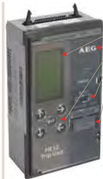
Fig. 2.1 LCD screen Battery Compartment KEY pad AUTO/MAN reset choice Full Range Rating Plug
