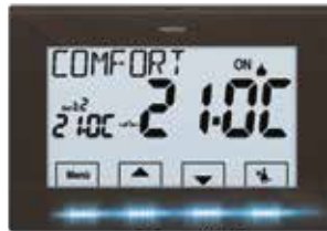
Between 18,1 °C and 21 °C the keys light up in blue indicating optimal consumption
